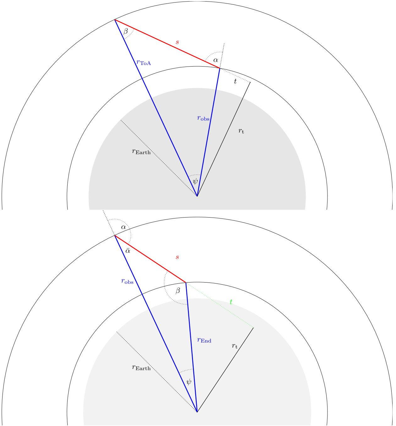
Figure 22: Geometry of uplooking (left) and downlooking (right) path: The observer is looking upwards (downwards) with an angle \alpha from the zenith along the line-of-sight (red).
