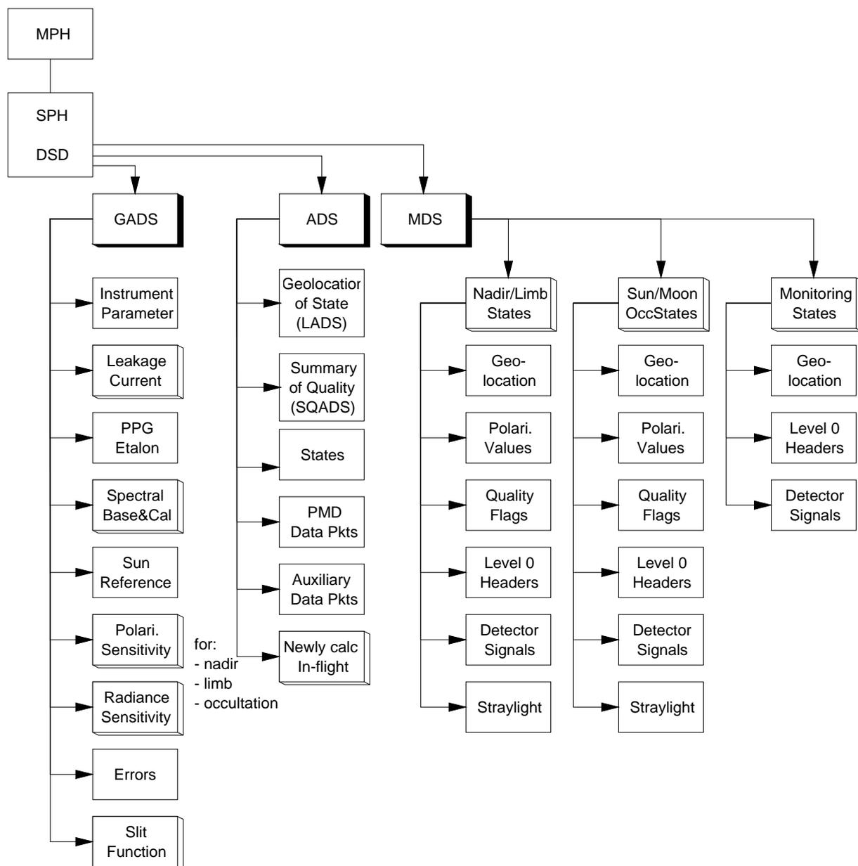
**Figure 3: Schematic Structure of the Level 1b Product**
