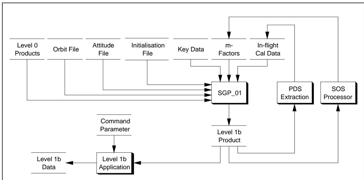
Figure 1: SCIAMACHY Level 0 to 1b Processing Overview
