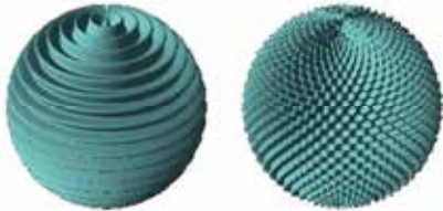
Chebyshev particles with 2D (left) and 3D (right) surface geometry used to model light scattering on particles with a small-scale surface roughness
