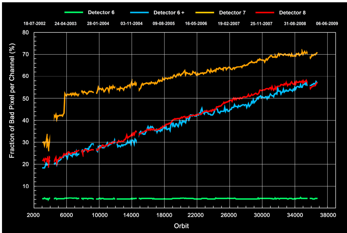
Fig. 6-9: Degradation of the pixel quality in the SWIR channels. The number of bad pixels is continuously increasing. For comparison, the first half of channel 6 is illustrated which consists of a material being more robust in the space environment and is thus much less subject to degradation. (Courtesy: SRON)
